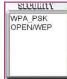
The WIFI Security List Box gives the user information about each of the SSID's security details, whether the security is WEP, WPA or OPEN. For example, in the screen above (fig. 2.9.9), the user can tell that the SSID 'BPC' is WPA secured, hence requiring a password in order to connect to that WIFI Network.
