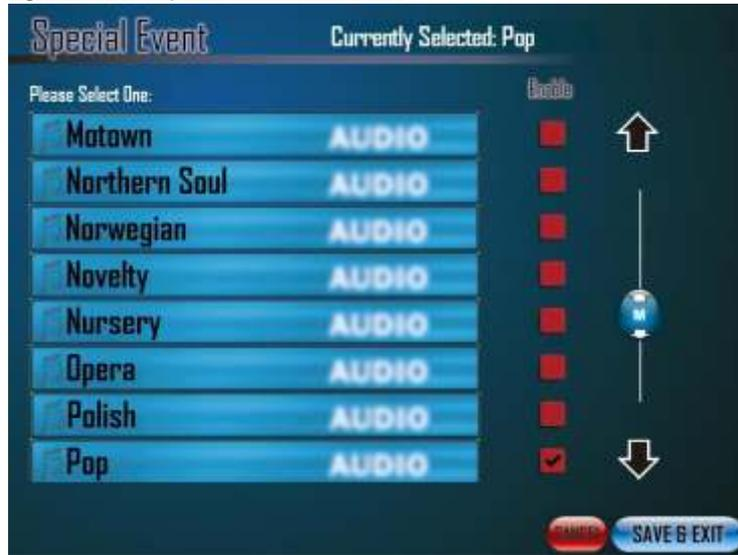
If you wish to control the special events on the Jukebox (which will display a button on the Jukebox main menu screen in the top left hand corner - see fig. 2.12.4) in the ADMIN section of the Service Mode Main Menu screen (fig. 2.12) you will need to enter **EVENT** for the password and then press the LOGIN button. This will display the screen as displayed above.
