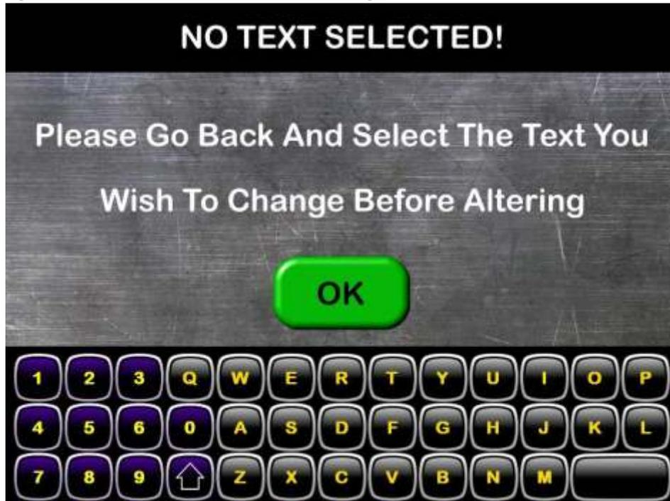
This error message is displayed if no text field is highlighted in the Preview Window (fig. 1.8.8.2) and the user enters the text in the Text Window and presses the ADD button (fig. 1.8.8.4). To clear this message, the user simply needs to press the OK button and the screen will revert to its previous state before the error message appeared.
