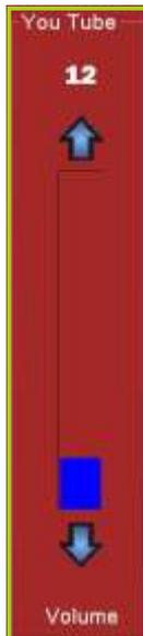
The **YouTube Volume** box, if the Kit is installed, (fig. 2.6.3) has only one bar (its own separate speaker) with the option to set the maximum volume limit of the YouTube feature to anything from 0-79. They can be adjusted by using the **Up** and **Down** arrows on each bar.
