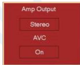
The settings in fig. 2.6.5 allow the user to change the amplifier settings for the Jukebox. The **Amp Output** can be changed between **Mono** and **Stereo** by clicking the button, the **AVC** (Automatic Volume Control) can be changed between **On** or **Off** by clicking the button. The default settings are: **Mono**, **On** respectively.
