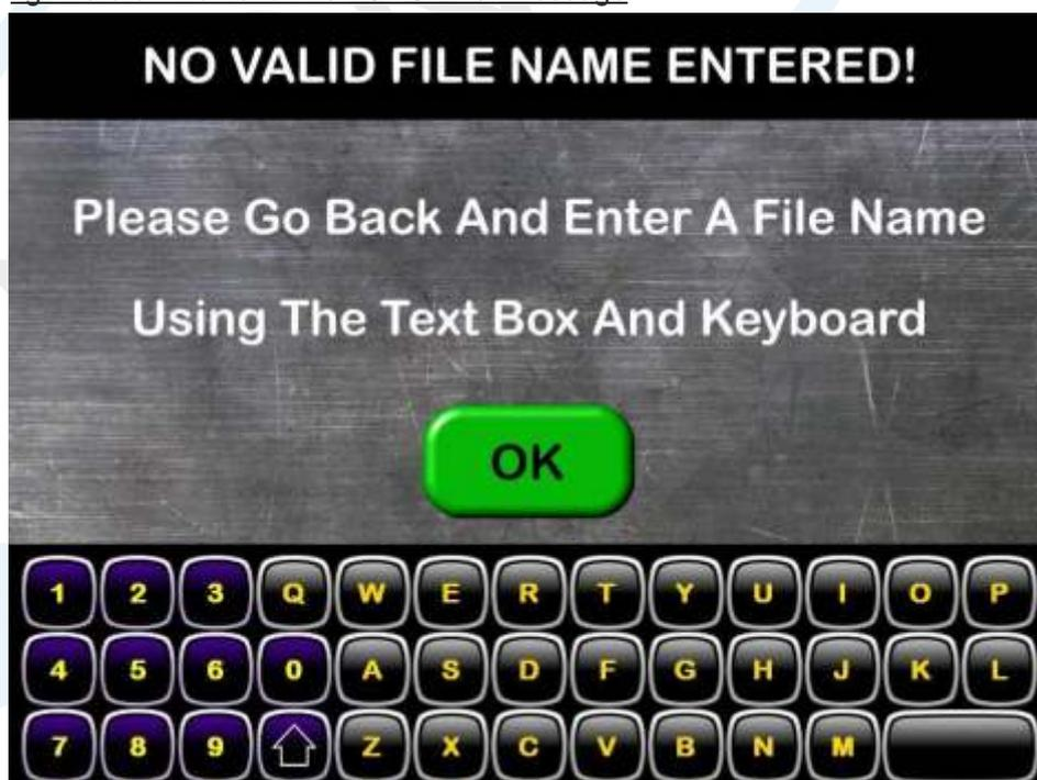
This error message is displayed If the user presses the Save button (fig. 1.8.8.1) and the Text Window is blank (fig. 1.8.8.4). To clear this message, the user simply needs to press the OK button and the screen will revert to its previous state before the error message appeared.
