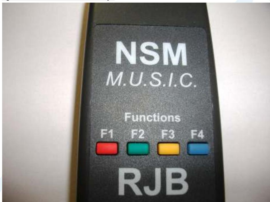
To access the Special Features Log In screen, the operator needs to press the F3 button, which will show the Jukebox Aux Mode screen (fig. 1.8.1), then the operator will need to press the F4 button to arrive at the Special Features Log In screen (fig. 1.8.2).
