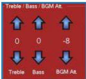
The settings in fig. 2.6.4 allow the user to set equalizer settings for the Jukebox. The **Treble** can be changed from -14 to 14, the **Bass** can be changed from -14 to 14 and the **BGM Att** can be changed from -36 to 0. These are all altered by using the **Up** and **Down** arrows on each option. The default settings are: 0, 0, -8 respectively.
