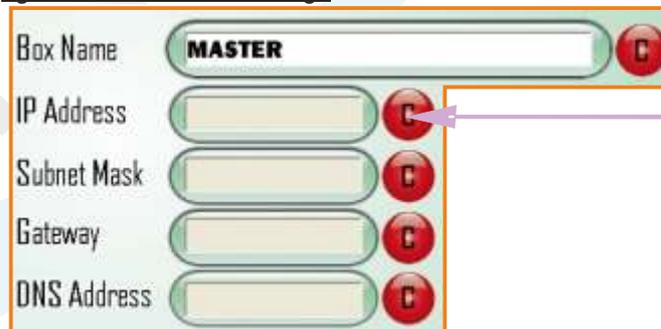
The 'C' Button clears the selected field ready to accept new text/numbers if the **Static IP** and/or the **Static DNS** button is active.
