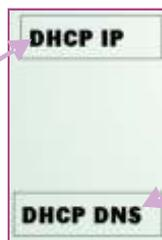
The **DHCP DNS** (Domain Name Server) Button greys out the **DNS Address** field to allow for automatic detection and connection. If the user presses the **DHCP DNS** button, the field becomes active and the text on the button changes to read **Static DNS**. This allows the user to enter their own DNS settings. (see fig. 2.9.4).
