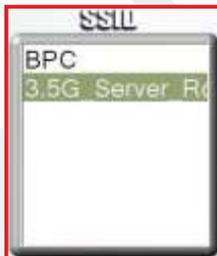
The WIFI SSID List Box displays a list of all the WIFI networks in range by it's SSID (Service Set IDentifier). If your network does not appear in the list, press the Refresh button (fig. 2.9.9.5).
