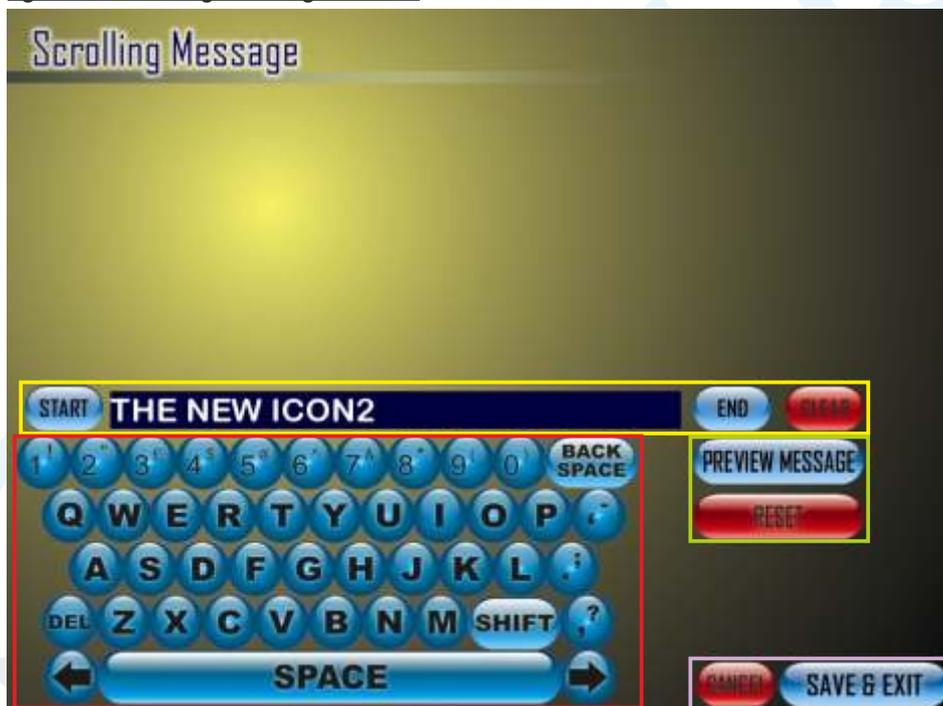
The Scrolling message can be altered to any message the user wishes by using the **On-Screen Keyboard** (fig. 2.3.1) which is a fully functional touchscreen keyboard designed to allow users to enter text in the **Scrolling Message** text box and any field that requires text input in any further **Service Mode** screens. The On-Screen Keyboard performs the same basic functions on all of the **Service Mode** screens that have need for it.
