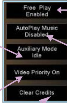
The **Auxiliary Mode** Button enables the auxiliary inputs on the Jukebox so if no music is being played on the Jukebox at the time the user can add an external source (i.e. hi-fi) to the auxiliary inputs, which will play music. It toggles between **Idle** and **Off**.
