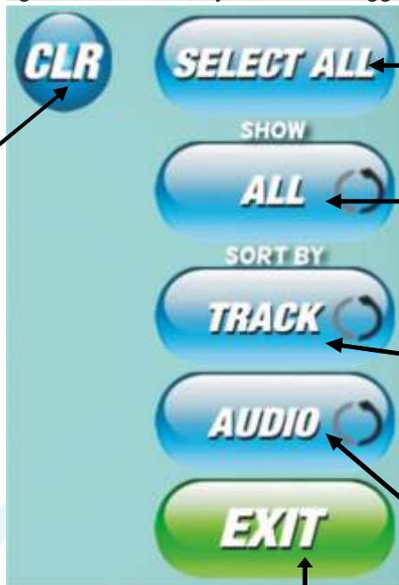
The CLR button, when pressed, clears all the text that is in the Text Box that the user has typed in using the on-screen keyboard.
