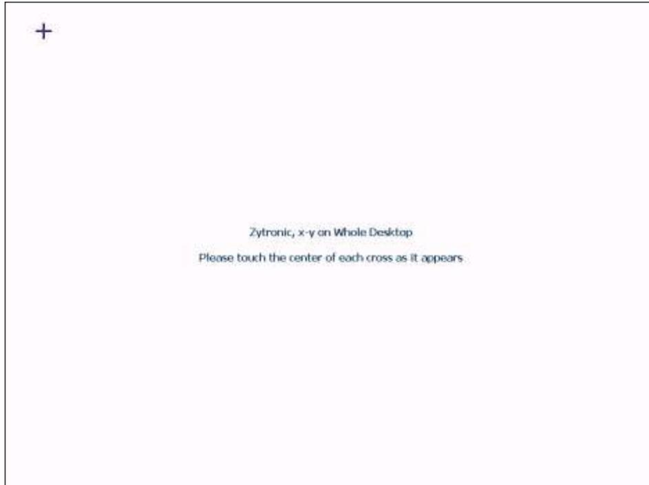
The screen above shows what happens when the user presses the **Screen Calibration** Button. When the button is pressed this new screen appears allowing the user to set up the touch screen, or to re-calibrate the touch screen after it has not been functioning as well as it should.
