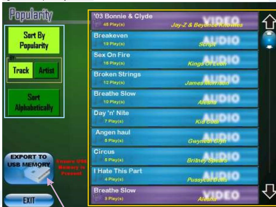
The **Export To USB Memory** Button saves the Popularity List as a .csv format which can be opened in Microsoft Excel for future Reference. Next to the button is a little reminder to the user to make sure that they have inserted a USB Flash Memory Stick. Any screen within the **Service Mode** which has this button will perform the same function.
