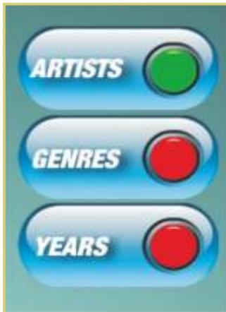
The 3 buttons opposite the list view allow the user to search for tracks in 3 different and independent databases (Artists, Genres or Years). The current selected database of tracks being viewed can be distinguished by the Green LED, the Red LED means that the others are not selected but can be when pressed, disabling the currently selected database of tracks.
