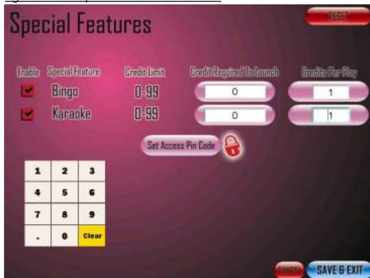
If you wish to control the special features on the Jukebox (Bingo & Karaoke functions) in the ADMIN section of the Service Mode Main Menu screen (fig. 2.12) you will need to enter **BINGO** for the password and then press the LOGIN button. This will display the screen as displayed above.
